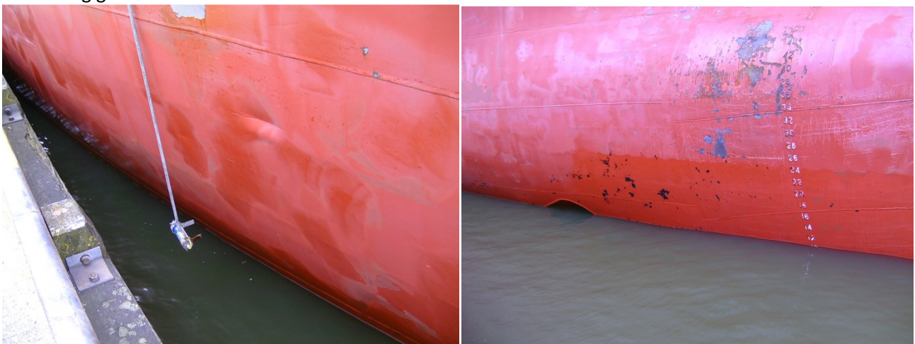
On these photographs, you'll see the hull around where the ultrasound head was placed. The paint is 9 months old and, within that period, the hull was not cleaned or touched up, but still looks new.
